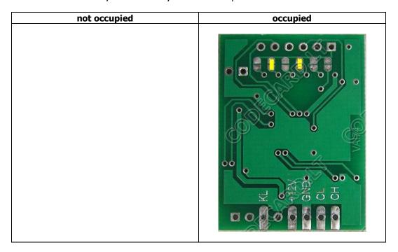
14. Renault CAN bus emulator for instrument cluster repair
